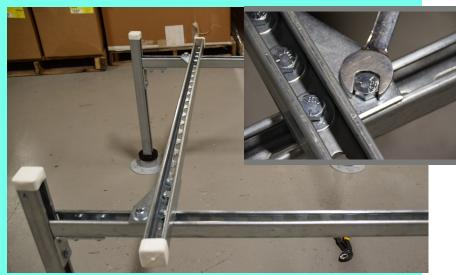
INSTALL VINYL END CAPS AND ATTACH UNIT TO ELEVATED MECHANICAL SUPPORT STAND AND MAKE ANY ADJUSTMENTS FOR LEVELING
