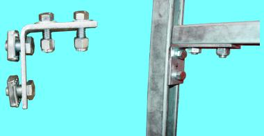
ATTACH SUPPORT RAIL (LONGER STRUT PIECE IF DIFFERENT SIZES) TO BRACKET, CHANNEL SIDE UP, SLOTTED SIDE DOWN, USING BOLT, NYLOCK NUT AND FLAT WASHER.
