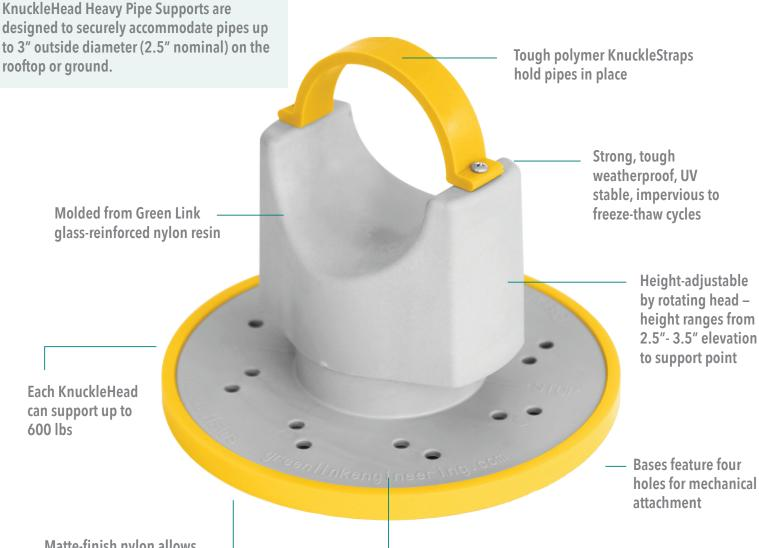
Matte-finish nylon allows bonding with adhesive
