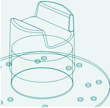
The KnuckleHead Support System serves two critical functions: as a load-bearing system, it delivers the necessary support for pipes, struts, pavers and related roof-mounted equipment. As an attachment system, it provides stability under conditions of wind uplift and seismic events. The tables below summarize important data with respect to the load-bearing and uplift resistance capabilities of installed KnuckleHeads.
