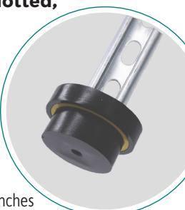
**The system provides three layers of protection against leaks:** Adhesive is applied to the base for bonding to the roof membrane and to the collar interior following attachment. The heat-sealed patch provides the third layer of protection.
