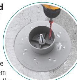
**KnuckleHead Stanchions are composed of slotted, galvanized steel** (hot-dipped and stainless steel are available on request) with an over-molded, threaded coupling that attaches to the center bolt of the KnuckleHead. Stanchions can be used to elevate equipment from 6 inches to 24 inches above the mounting surface. Each head can support up to 600 pounds.
