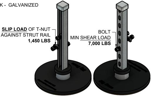
ASSEMBLY TORQUE RANGE OF NUTS AND BOLTS: 60-80 FOOT-POUNDS
