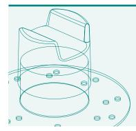
The KnuckleHead Support System serves two critical functions: as a load-bearing system, it delivers the necessary support for pipes, struts, pavers and related roof-mounted equipment. As an attachment system, it provides stability under conditions of wind uplift and seismic events. The tables below summarize important data with respect to the load-bearing and uplift resistance capabilities of installed KnuckleHeads.
